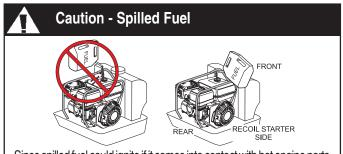
Since spilled fuel could ignite if it comes into contact with hot engine parts, **ALWAYS** pour fuel from the **recoil starter side** of the compactor. Allow engine to **cool!** before refueling. Wipe up any spilled fuel immediately.
